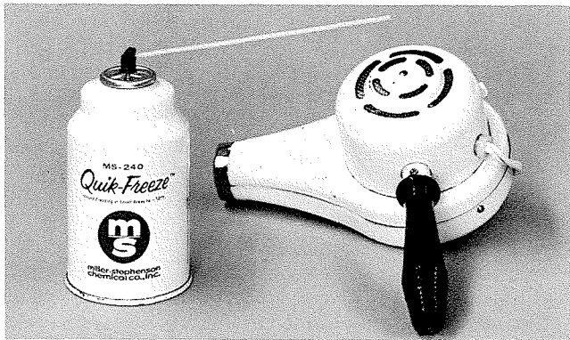
Elusive intermittents are often nailed by using circuit cooler and a hair dryer.
