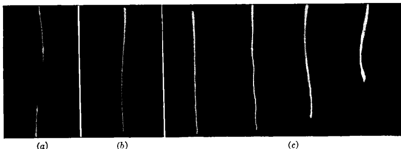
FIG. 9-12.—Typical sweep distortions. (a) Defocusing and curvature due to sectional oscillation of the deflection coil. (b) Curvature produced by oscillations in a toroidal deflection coil. (c) Sweeps showing effect of insufficient recovery time.
