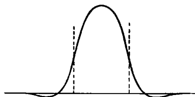
FIG. 8-28.—Axial field distribution of an air-core coil. Ends of the coil are marked by dashed lines.
