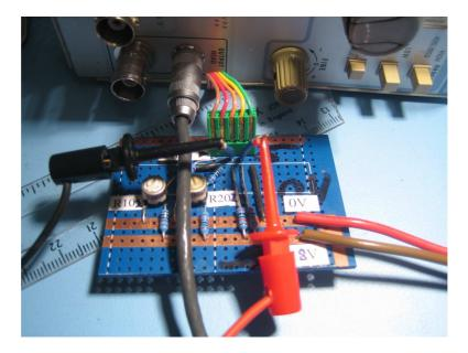
The first thing you will need to do is connect the calibrator to a lab PSU set for 18.00V (make sure you get the polarity the correct way round). Then there is a "one time action" to calibrate the calibrator which involves adjusting R102 and R202 as described on the schematic page.
