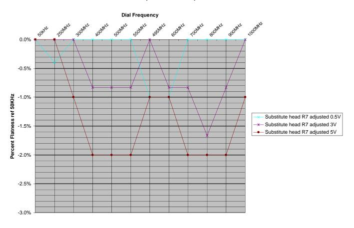
Leveller Output flatness compared to 50kHz
