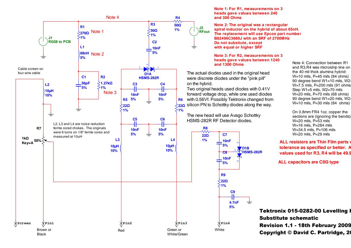
the 40 mil thick alumina hybrid: W=10 mils, P=45 mils (84 ohms) 90 degree bend W1=10 mils. W2=7.5 mils W=7.5 mils, P=200 mils (91 ohms) Step W1=5 mils, W2=70 mils W=20 mils, P=70 mils (68 ohms) 90 degree bend W1=20 mils, W2=10 mils W=10 mils, P=30 mils (84 ohms)
