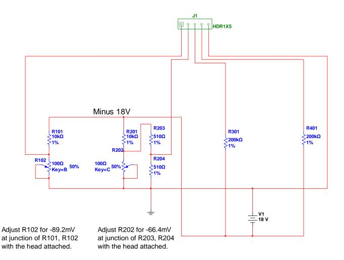
Adjustments of R102, R202 are one time adjustments to the calibration circuit.
