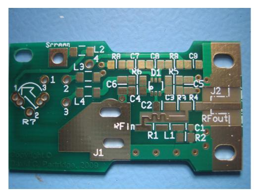
The PCB is designed to be used either in your own case; or in the original Tektronix housing (if you have a dead levelling head). To use it in your own case I have provided pads for an SMA bulkhead end launcher at the right hand side. In this case, as well as the SMA end launcher you will need an SMA male to BNC male adapter.
