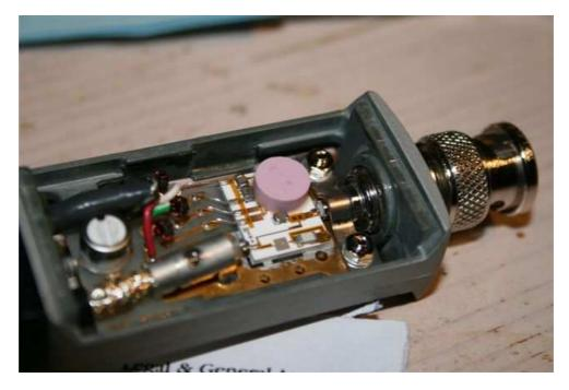
The basic design is an RF power splitter, and a voltage doubler peak detector. The diodes for the detector are under the pink isothermal cover at the top right of the hybrid, as are the reference diodes and a few other components.
