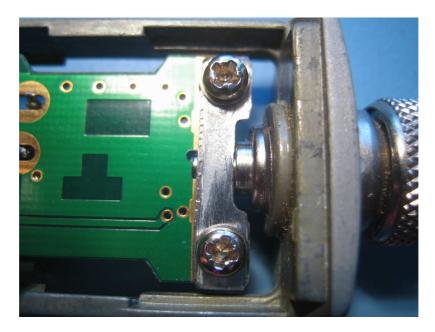
All that remains is to connect the 4 core cable to connection points 1 to 4, solder the input coax screen and use a fine wire to connect the centre core of the input coax to the pad next to R1, and finally to solder the centre connector of the output connector:
