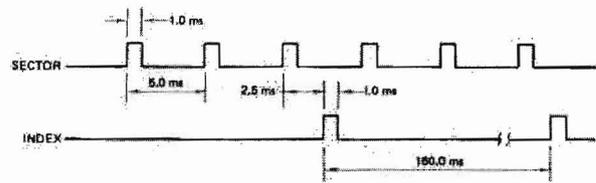
Fig. 2 (a) Timing relationship between the index and sector pulses.
