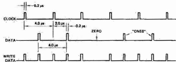
Fig. 2 (b) WRITE data timing and signal waveforms.
