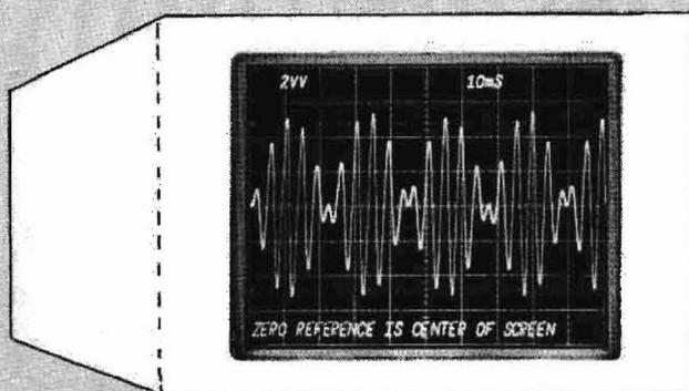
The readout in this photo was programmed by the computer in a Digital Processing Oscilloscope system. The double V indicates the waveform is the resultant of two voltage signals multiplied together.
