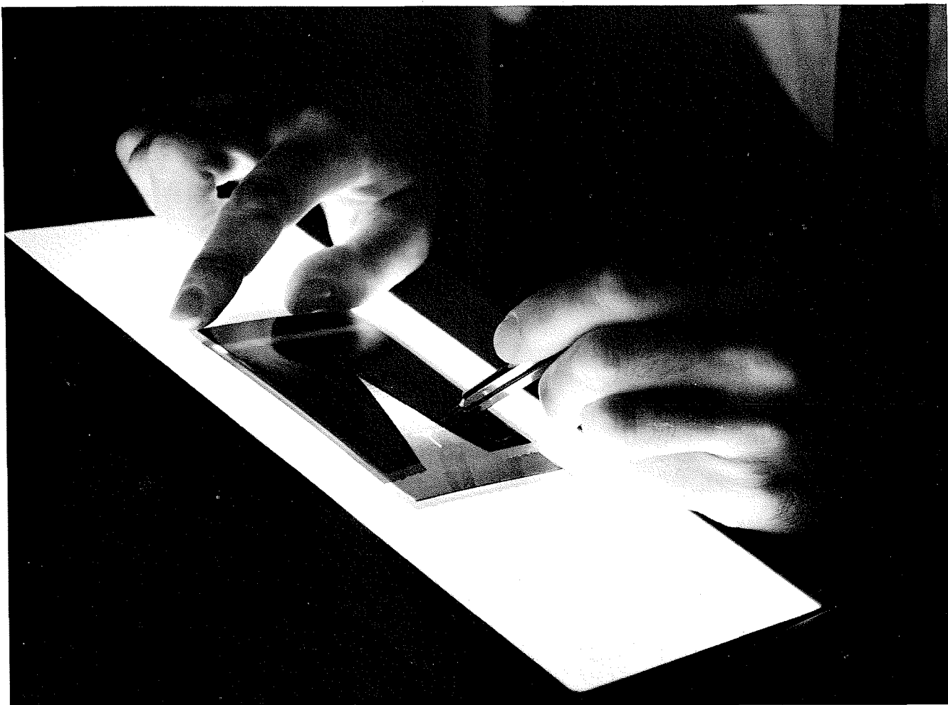
Fig 1 Determining writing speed from a backlighted photograph. Note the use of a mask to cover the peaks of the waveshape.
