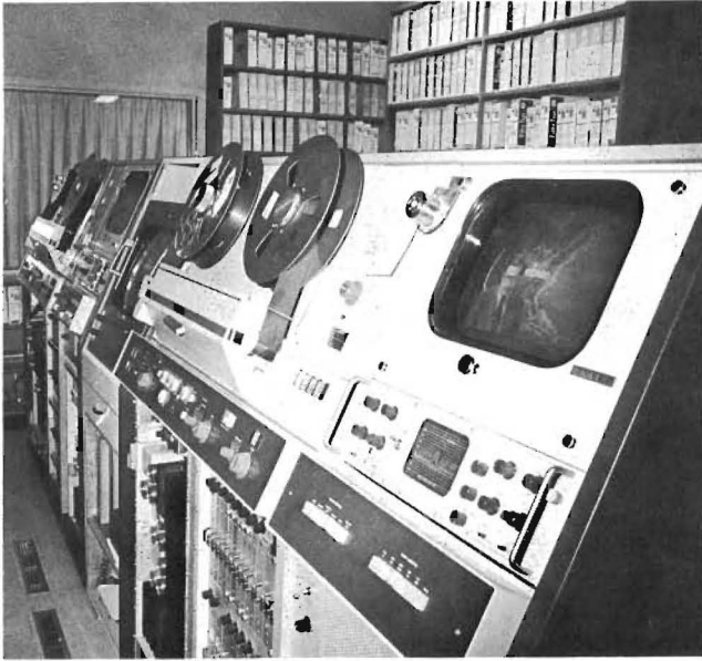
TEKTRONIX Waveform Monitors are an integral part of these broadcast video tape recorders. Photo courtesy of KGW
