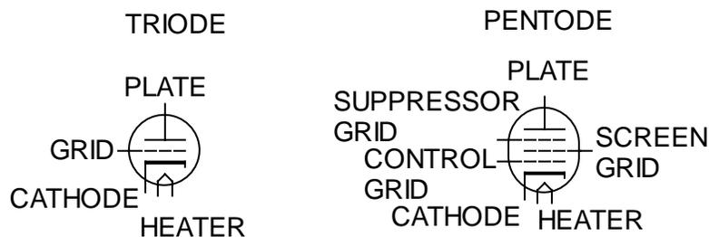
**Fig. 4: Schematics Used For Triode And Pentode With Connections**
