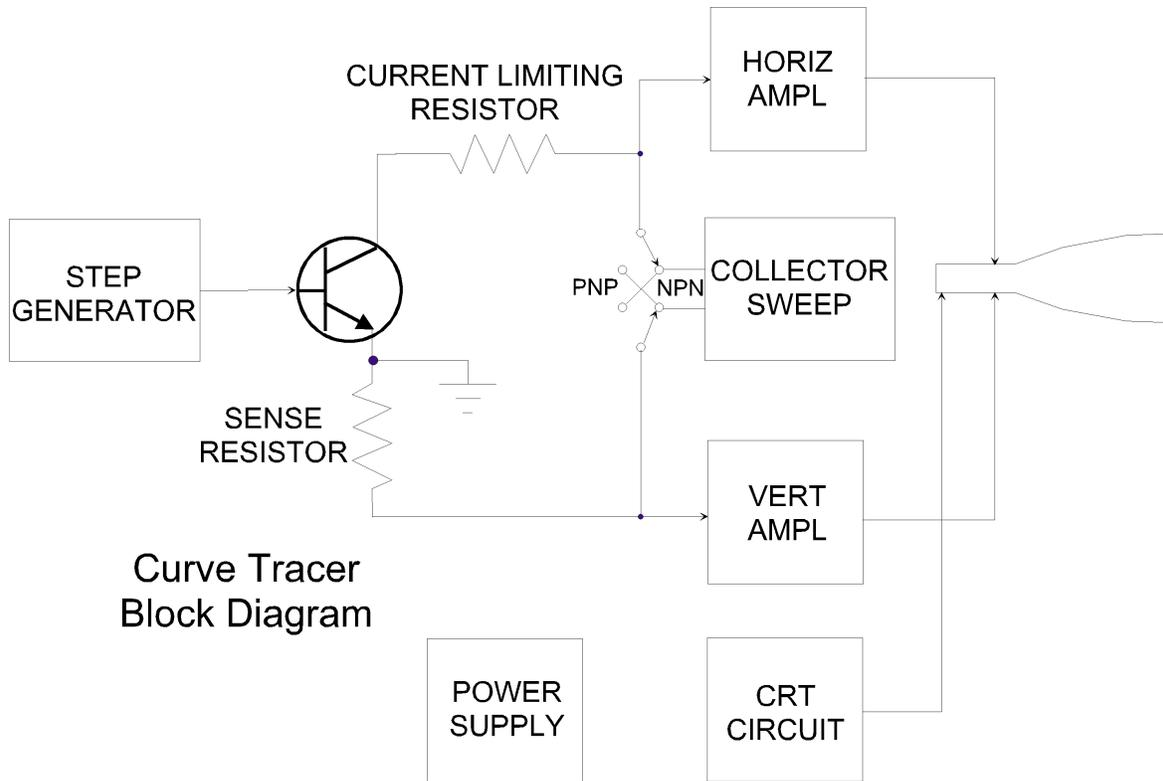
**Fig. 2: Block Diagram Of The 575 Curve Tracer**
