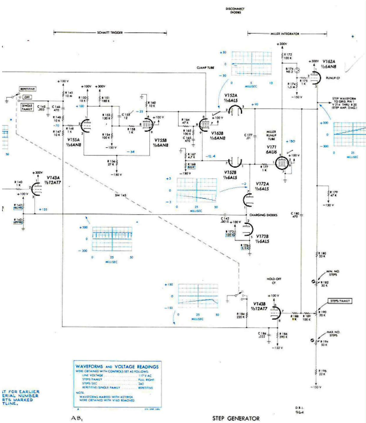
**Fig. 3: The Tek 575 Step Generator Circuit Diagram**
