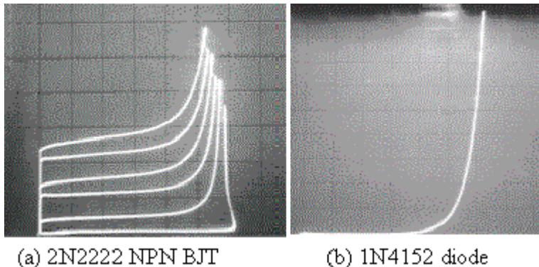
**Fig. 1: Curves Of (a) npn Bipolar Junction Transistor (BJT), (b) Diode**
