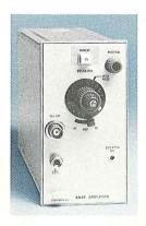
The 5A45 Single-Trace Amplifier provides the 5400-Series Oscilloscope with 60 MHz bandwidth and deflection factors from 1 mV/div to 10 V/div (25 MHz bandwidth below 5 mV/div). Crt readout of the deflection factor is included.
