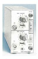
The 5A38 Dual Trace Amplifier is designed for use in the 5400-Series Oscilloscopes. It provides two input channels with 35 MHz bandwidth and deflection factors ranging from 10 mV/div to 10 V/div. Operating modes include channel 1 only, channel 2 only (normal or inverted), dual trace (alternate or chopped), and added. Crt readout of the deflection factor is included in the 5A38.
