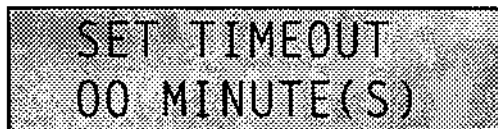
Figure 3-32. Setup Screen No. 20 - Set Timeout
