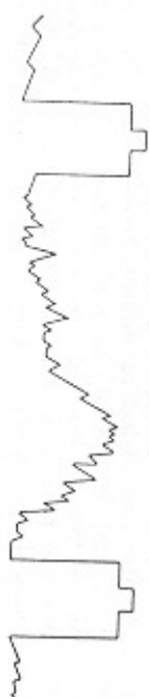
Figure 4—Normal Video and Sync Signal.
