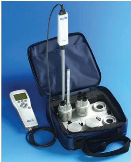
Example of salt solution chamber for humidity instrument calibration
