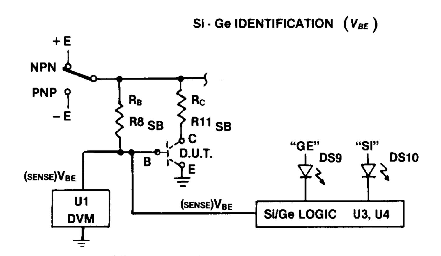
Figure 6. Si-Ge Identification SI/GE LOGIC (SENSE) VBE GE **READ OUT** GE CONDITION U4 BLANK  $|V_{BE}| < 2V$  $.1V < |V_{BE}| < .4V$ Ge Н .4V  $.4V < |V_{BE}|$ Si Figure 7. SI/Ge Logic
