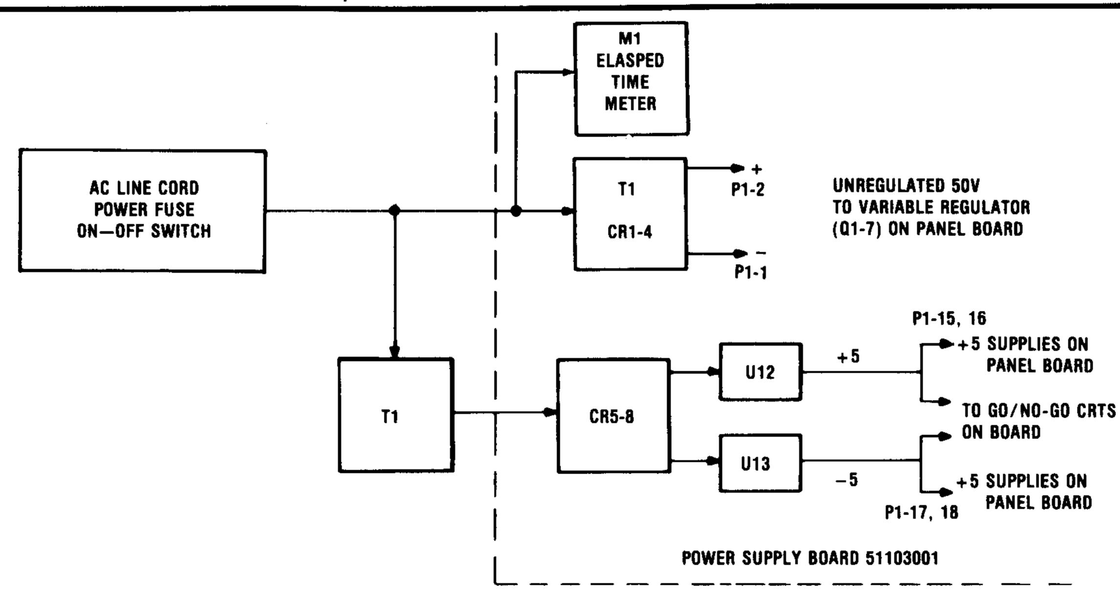
Figure 4. Power Supply Block Diagram
