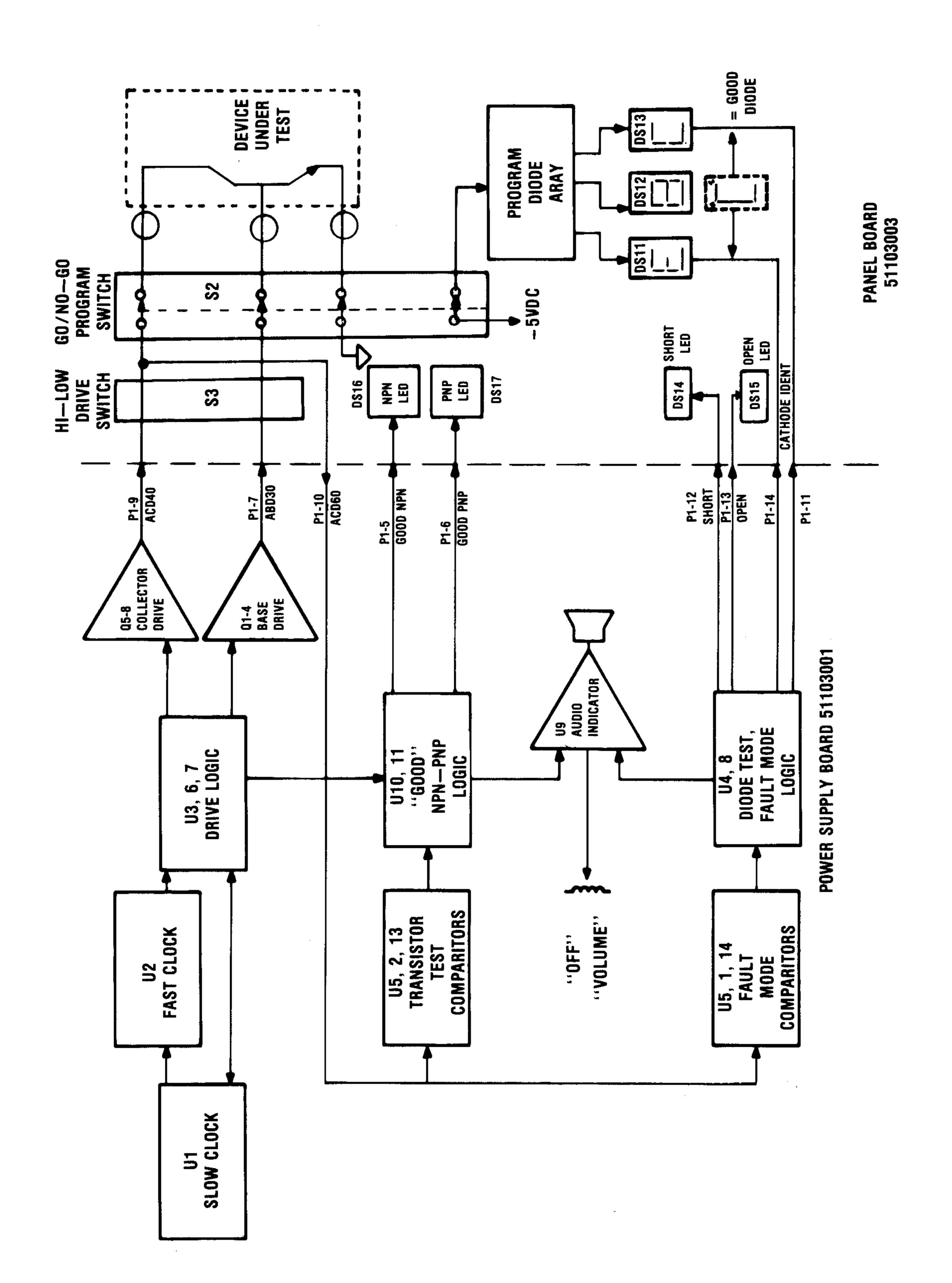
Figure 5. Go/No-Go Block Diagram
