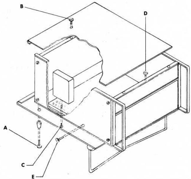
Figure 5-1. Disassembly
