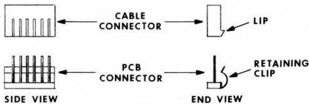
Figure 5-3. Connector Alignment
