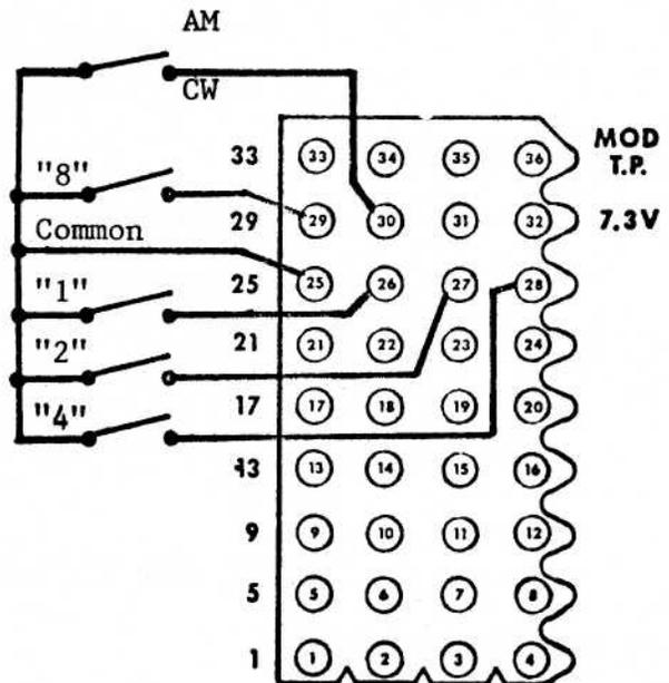
Figure 8/1B-1. Plug Connections
