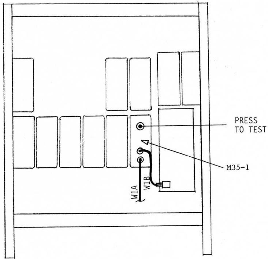
Figure 8/3-2. Top View, RF Circuit Breaker Location
