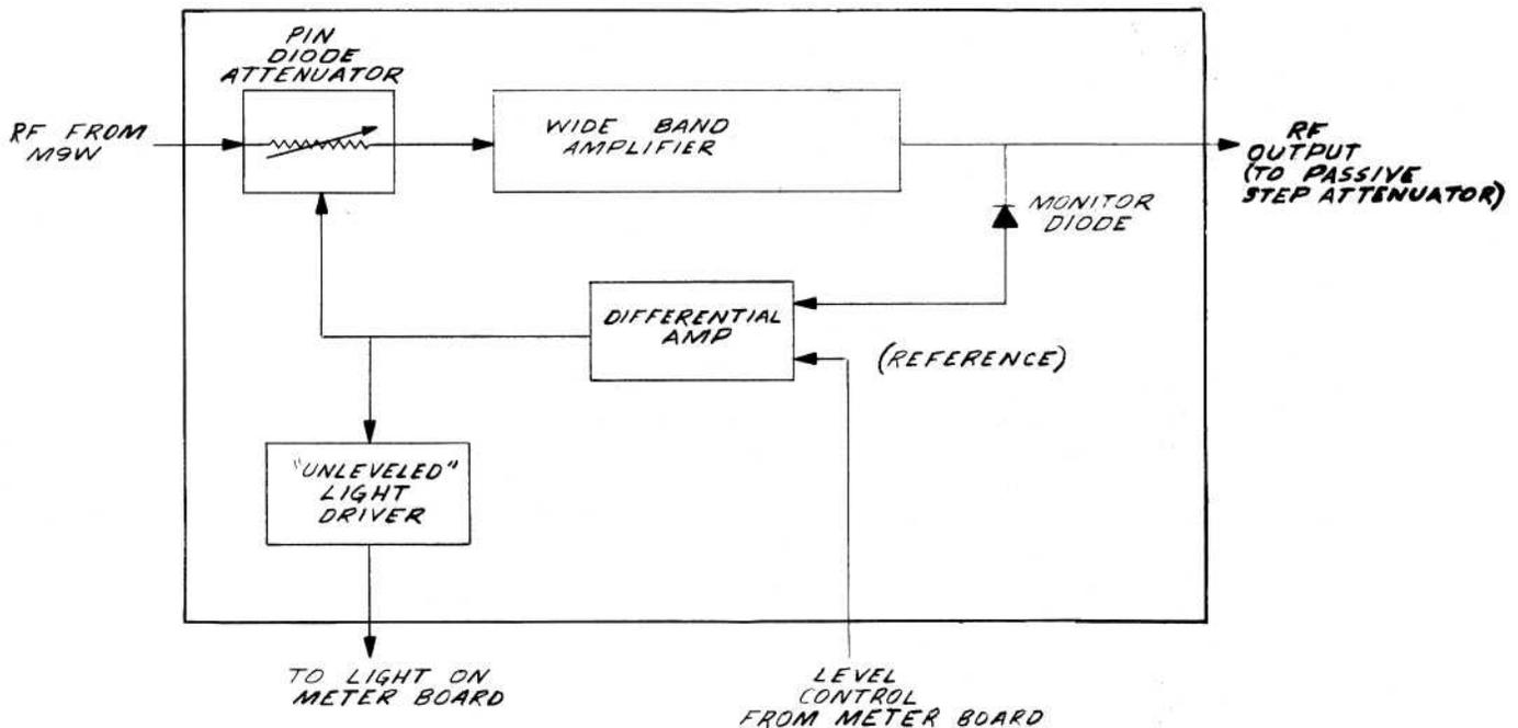
Figure 3-13. M10W - Output Amplifier
