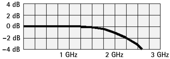
Figure 3 Typical frequency response with short pin ground clip
