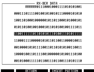
Fig. 10.15: The BER data field shows the complete bit sequence output by the Communication Test Set.
