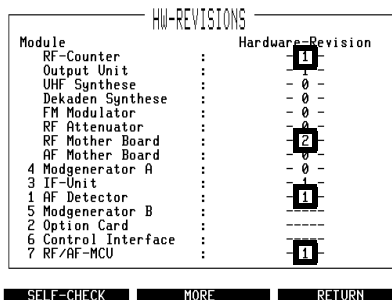
Fig. 10.2: If the mask shows smaller entries for the marked fields, you will have to update the corresponding stage.
