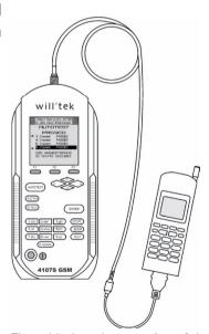
The cable-based connection of the test unit is the ideal choice for precision measurements.
