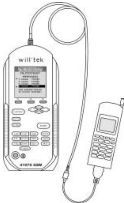
Cable-based connection of the test unit is the ideal choice for precision measurements.
