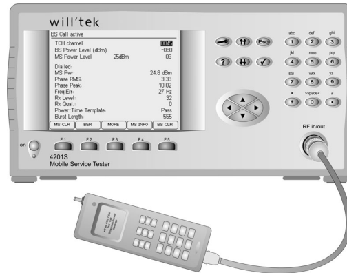
Cable-based connection of the test unit is the ideal choice for precision measurements.
