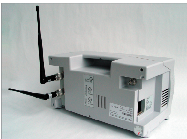
Figure 3: The back of the 4208 shows separate connectors for radio frequency input and output. Isolation between receive and transmit paths can be improved by arranging the two antennas in a 90° angle
