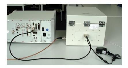
3 Plug the Bluetooth adapter into the D-type RS-232 connector inside the 4921 RF Shield.
