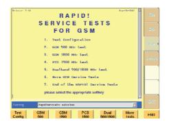
The RAPID! Service Test software provides easy access to the most common tests required in a service environment. Navigation is made straightforward through the use of softkeys.
