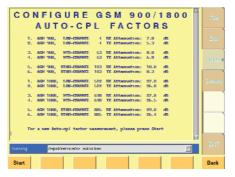
After the Autocalibration feature has measured all the results along with the "golden" mobile the 4400 presents the results as they are stored under the type approval code (TAC). These values will be taken as reference once the same type of phone is tested with the 4400 Service software.
