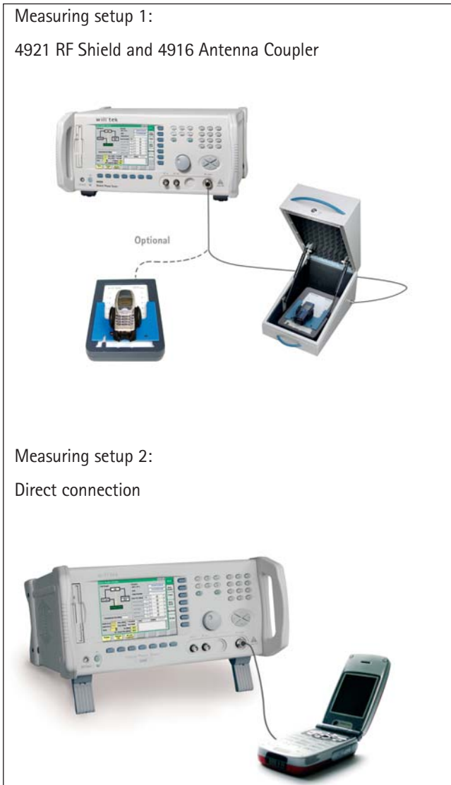
Figure 2: Measuring setup variants for final testing the TD-SCDMA wireless terminal
