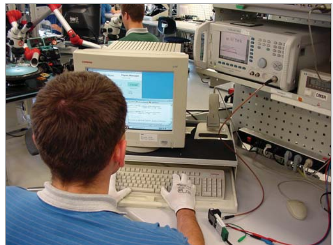
Figure 1: 4403 Mobile Phone Tester – the ideal tool for service centres and the repair loop in production
