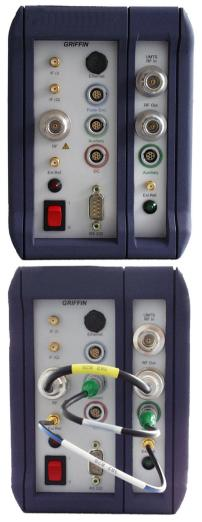
If you want to use the Griffin in the frequency range from 2000 to 2200 MHz (UMTS Down Converter Option) or in the 300 to 500 MHz range (Up-Converter Option):
