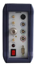
Antenna input The antenna should be chosen to suit the frequency band of the Griffin in use (800 to 1000 MHz or 1700 to 2000 MHz). It can be connected directly to the RF input connector or via a length of low-loss cable. The input is a conventional 50 W N-type.
