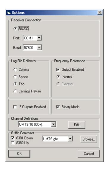
The Front Panel Software has various options that you can use to adjust how it operates. These options are recalled the next time you run the Software. To change the options choose Options from the Tools menu. This will give you a dialog box which has six sections as follows.
