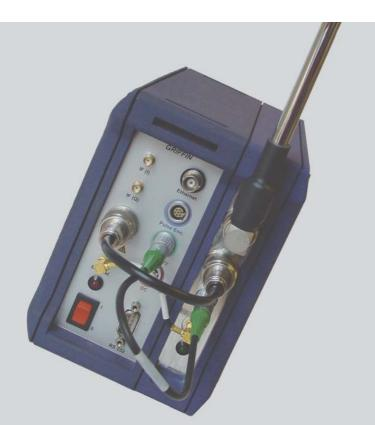
Measures radio systems in the 300 to 500 MHz band including TETRA, analog rail systems and CDMA 450 networks
