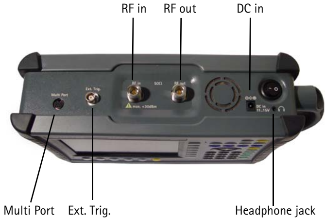
Figure 2 Connectors on the top of the 9102
