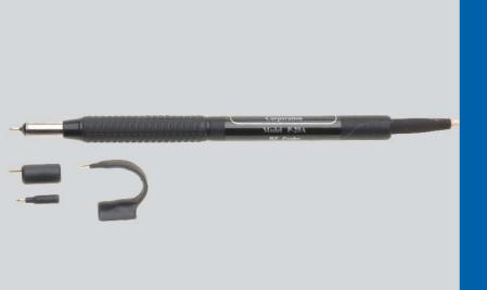
Bandwidth: 100 kHz to 4 GHz Low Distortion, Passive RF Design Light RF Loading Characteristics Internal 50 VDC Block 10:1 Voltage Ratio Rugged Design The 1205 RF Probe 20 dB is a passive 10:1 RF voltage probe with a 50 VDC block built in.
