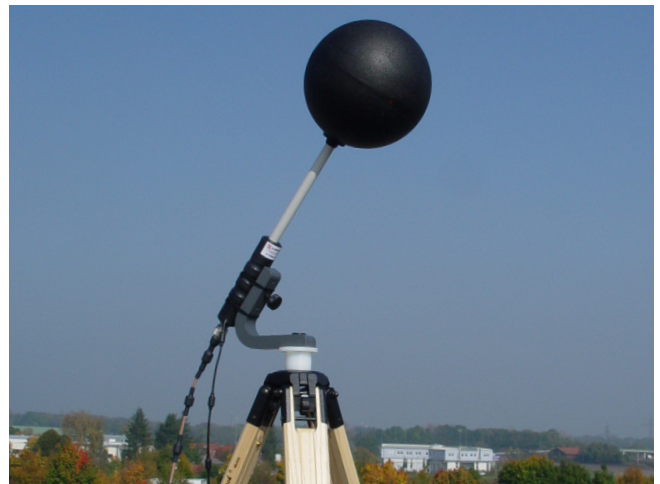
The 9102 with the 9171 Isotropic Antenna is a comfortable test solution for immission measurements.
