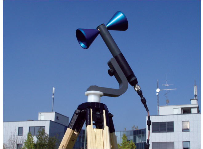
With biconical antennas, the same antenna pair is used to take measurements in different directions.
