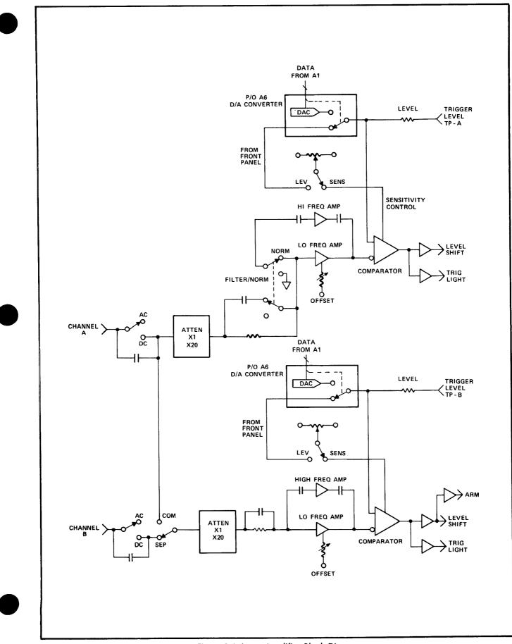
Figure 3-6. Input Amplifier Block Diagram
