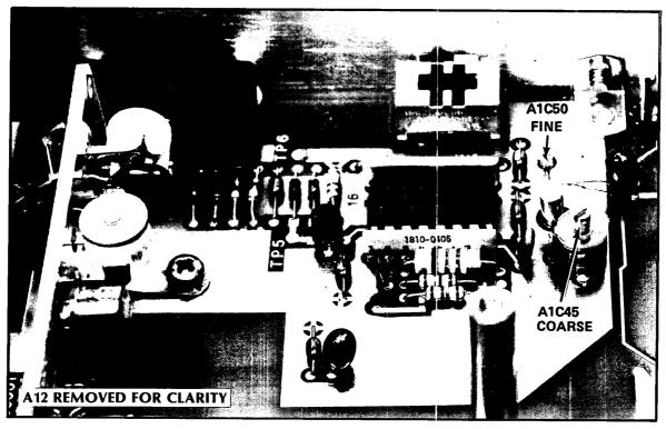
Figure 5-5. Injection-Locked-Multiplier Adjustment Location
