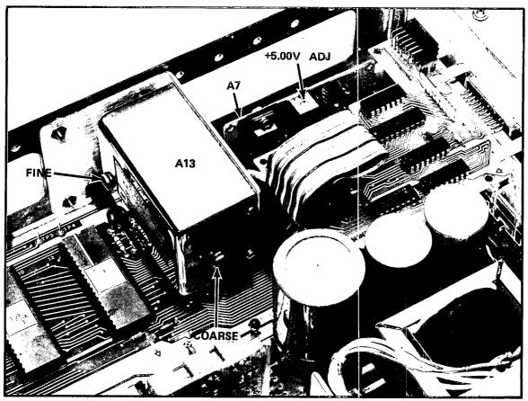
Figure 5-8. Option 004 Oven Oscillator Adjustment Location
