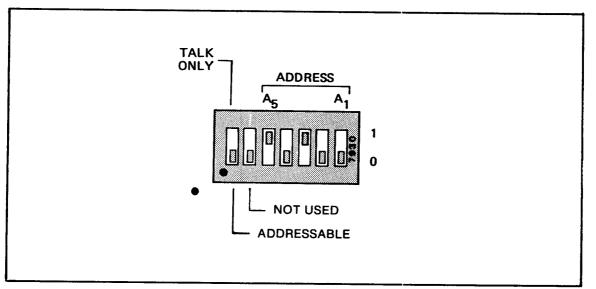
Figure 3-22. 5316A Address Switches (20)
