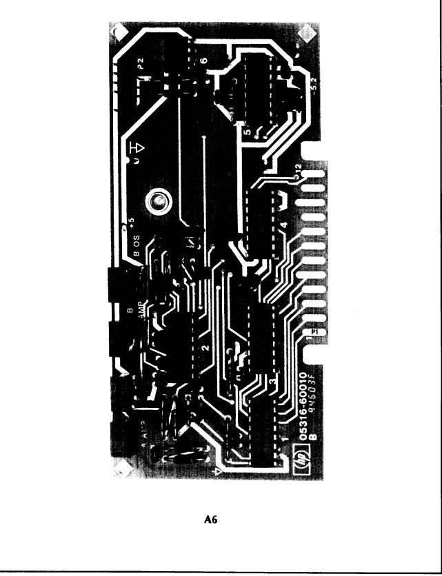
Part of Figure 8-9. A6 Digital-to-Analog Converter Assembly
