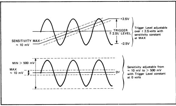
Figure 3-5. Trigger Level/Sensitivity Control
