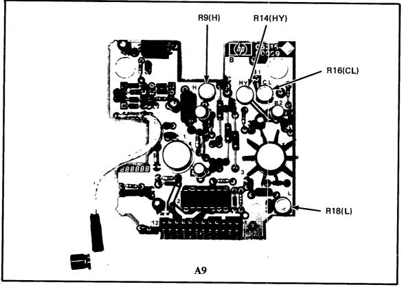
Figure 5-9. Channel C Adjustment Location
