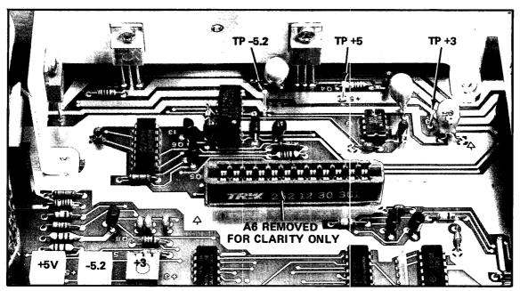
Figure 5-1. Power Supply Adjustment Location
