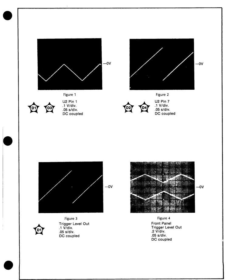
Part of Figure 8-9. A6 Digital-to-Analog Converter Assembly
