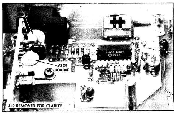
Figure 5-6. Internal Time Base Adjustment Location
