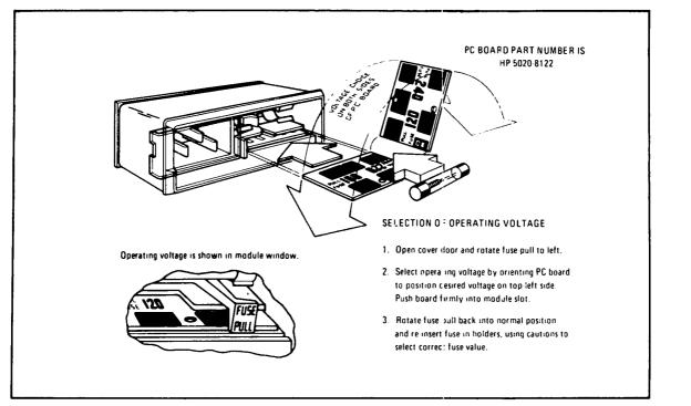
Figure 2-1. 5316A Line Voltage Selection
