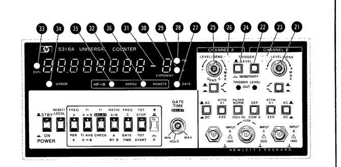
**LEVEL/SENS.** When in TRIGGER LEVEL, controls the voltage at which CHANNEL A input will trigger, variable over ±2.5 volts X ATTN setting. When in SENSITIVITY, varies the sensitivity from MAX (≈10 mV) up to 500 mV. In FREQ C, controls the input sensitivity for INPUT C from MAX (≈15 mV up to 650 MHz, 75 mV up to 1 GHz) up to MIN (20 dB NOMINAL).
