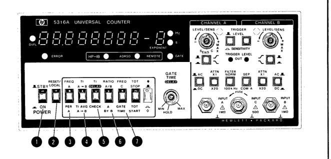
**STBY/ON.** Supplies power to entire machine in the ON position. Removes power from the voltage regulators when in the STBY (Standby) position.
