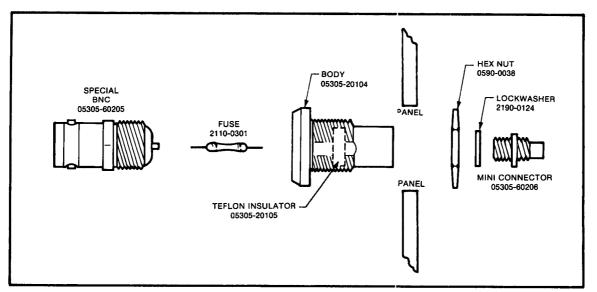
Figure 3-9. Details of Input Connector J1 and Fuse Mounting
