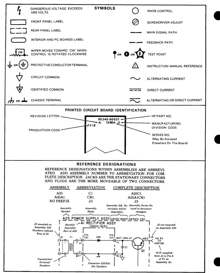
Figure 8-1. Schematic Diagrams Notes
