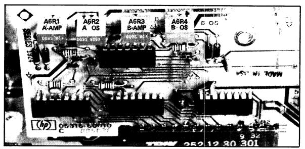
Figure 5-3. Digital-to-Analog Converter Adjustment Location
