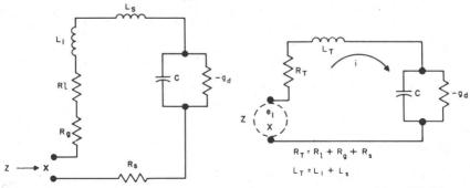
(A) SERIES CONFIGURATION OF AMPLIFIER OR OSCILLATOR CIRCUIT
