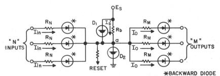
CHOW'S ANALOG-THRESHOLD LOGIC CIRCUIT
