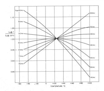
VARIATION OF NORMALIZED  $I_P$  WITH TEMPERATURE FOR DIFFERENT VALUES OF  $V_P$  FIGURE 2.3
