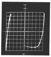
cessive series inductance in the test circuit. As the sweep goes through the negative conductance region, this inductance will resonate with the diode and circuit capacitances, making the circuit oscillate and causing a display as shown in Figure 7.2.
