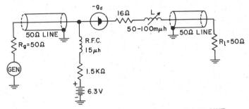
COMPLETE 100 Mc/s "SERIES" AMPLIFIER CIRCUIT FIGURE 3.14
