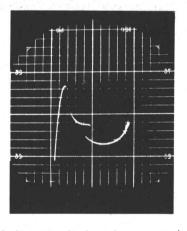
If the total circuit inductance (including the diode inductance  $L_s$ ) is kept at a minimum, this oscillation will not occur. Actually, if the circuit self-resonant frequency  $f_{xo}$  (circuit) is made larger than its cut-off frequency,  $f_{ro}$  (circuit), no oscillations can occur. To meet this criterion, the total circuit inductance must be smaller than:
