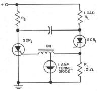
TUNNEL DIODE USED AS CURRENT SENSING ELEMENT IN SILICON CONTROLLED RECTIFIER CIRCUIT BREAKER
