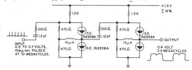
TUNNEL DIODE TWO STAGE COUNTER
