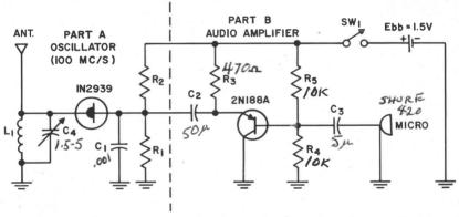
R<sub>1</sub> 22Ω -1/2 WATT C1 .OOI CERAMIC DISC.
