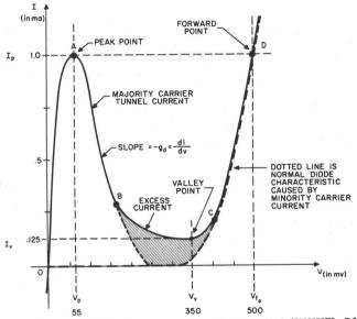
STATIC CHARACTERISTIC CURVE OF GERMANIUM TUNNEL DIODE
