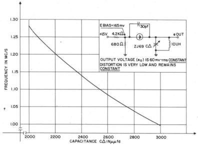
FREQUENCY TUNING BY MEANS OF  $C_{\Delta}$ FIGURE 4.9
