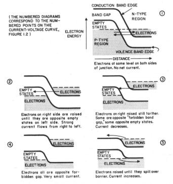
TUNNEL DIODE JUNCTION AT VARIOUS BIAS CONDITIONS
