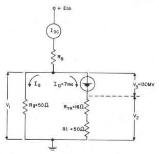
DC BIAS CIRCUIT FOR 100 Mc/s AMPLIFIER STAGE FIGURE 3.13
