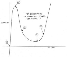
TUNNEL DIODE CHARACTERISTIC
