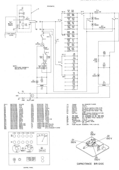
CAPACITY TEST SET CIRCUIT DIAGRAM
