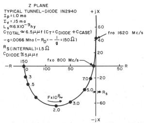
CHARACTERISTICS OF A TYPICAL TUNNEL DIODE FIGURE 3.6
