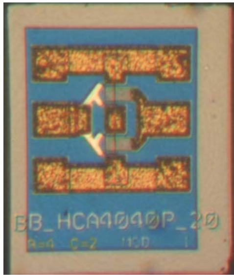
Fig. 5-9. Typical HEMT chip after scribe and break. (Note: all chips are inscribed with data identifying position on the wafer, gate number, and gate width)
