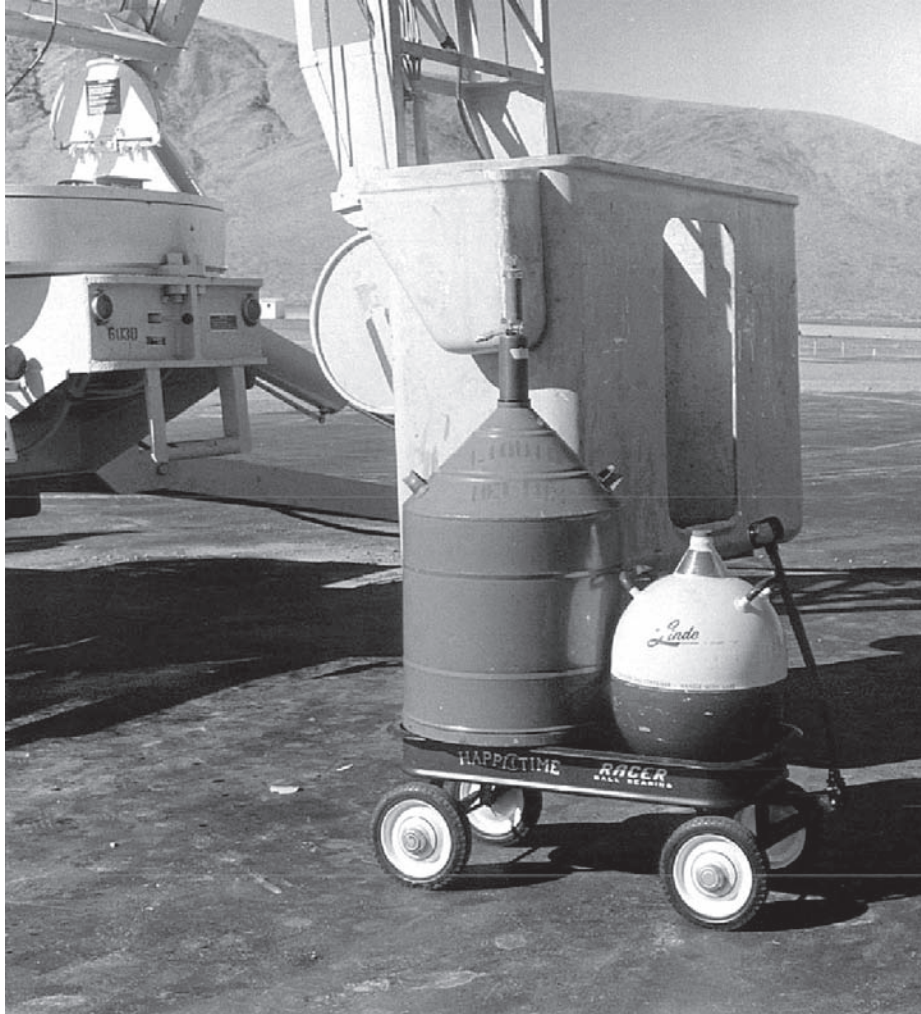
Fig. 4-4. Liquid helium and liquid nitrogen dewars on "HAPPYTIME RACER" utility vehicle with the cherry picker (High Ranger) and cherry-picker fiberglass basket in the background.
