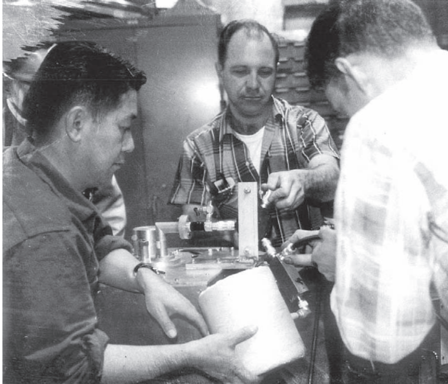
Fig. 4-5. Noise temperature measurement (manually switching between ambient and liquid nitrogen temperature loads) showing use of styrofoam container for storing liquid nitrogen.
