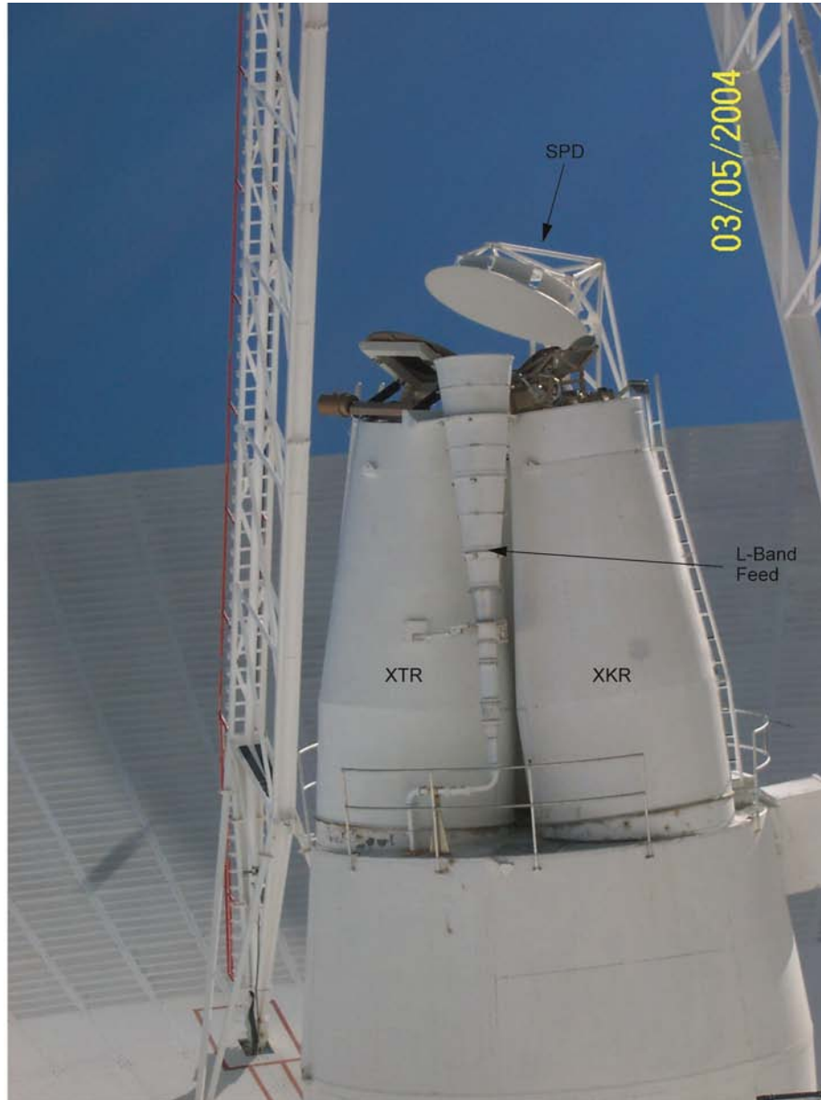
Fig. 2-1. Goldstone 70-m antenna tricones S-band polarization diversity (SPD) feedcone located behind the X-band/K-band radar (XKR) and X-band transmit/receive (XTR) feedcone.
