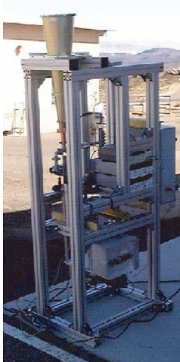
Fig. 7-3. 13.8-GHz microwave package TPR during testing prior to installation at DSS-13 at F_3 .
