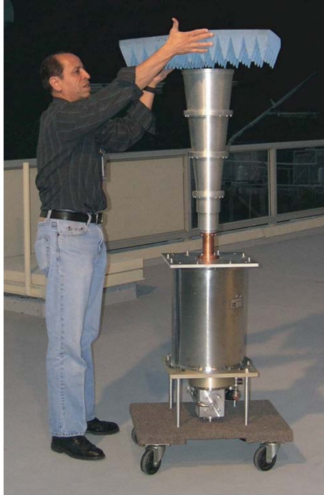
Fig. 2-21. X-band (8.5-GHz) calibrated feed and LNA system demonstrating a manual aperture load noise temperature measurement technique.
