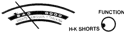
Fig. 11 — A short between the heater and cathode is indicated by a BAD reading.
