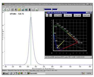
SpectroRadiometry & LED xy Chromaticity & Correlated Color Temperature (CCT)
