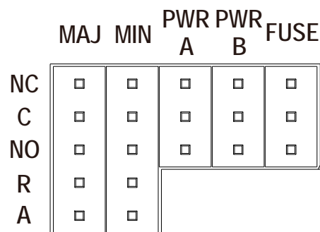
Figure 8 - Alarm Terminals on Rear of Panel
